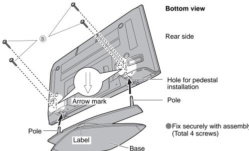
Fix securely with assembly screws B.
